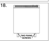
**19.** Check that the screws securing the heater to the wall bracket have been fully tightened.
