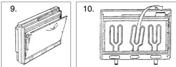
10. Remove one element to allow access for the back row of bricks. On the 24 remove the element to the right of centre, on the 18 remove the central element, on the 12 the left hand element should be removed.
